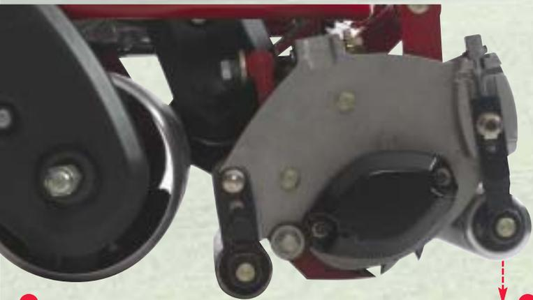
**THE CUTTING UNIT** sets back roller down softly first, then front, like an airplane landing, to prevent gouging.
