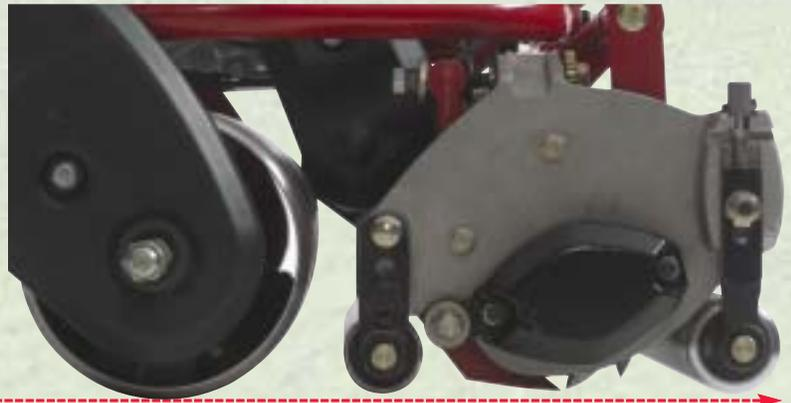
**THE UNIQUE POSITIONING** of two rollers tucked closer to the reel and rear drum means you're far less likely to mark an undulating green.
