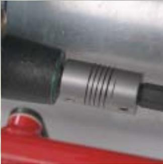
**FLEXIBLE DRIVE SHAFT COUPLERS** allow the cutting unit to flex on the center axis.
