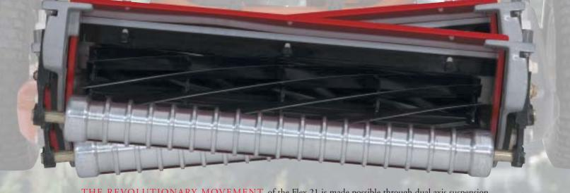
THE REVOLUTIONARY MOVEMENT of the Flex 21 is made possible through dual axis suspension and flexible drive shaft couplers. The individual traction and cutting units are attached at two center pivot points so the cutting head can pivot forward and back, and side to side around the bedknife centerline.
