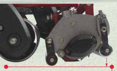
THE CUTTING UNIT sets back roller down softly first, then front, like an airplane landing, to prevent gouging.
