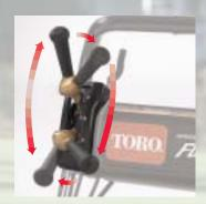
A DUAL-FUNCTION LEVER controls both the traction and reel. Plus a new clutch design makes it easy to engage the reel with a simple twist of the wrist.
