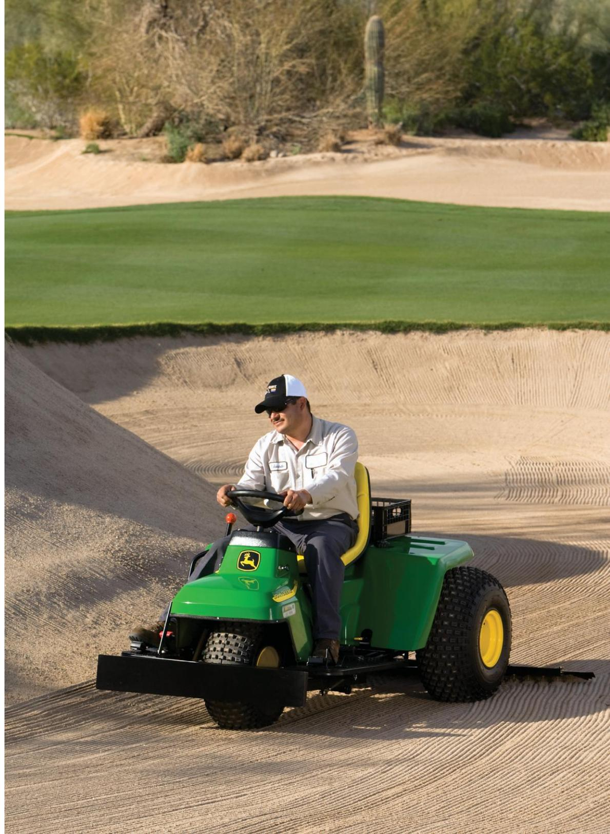
STEERING WHEEL HAS AN 8.4-TO-1 GEAR RATIO FOR EASY AND RESPONSIVE STEERING.
