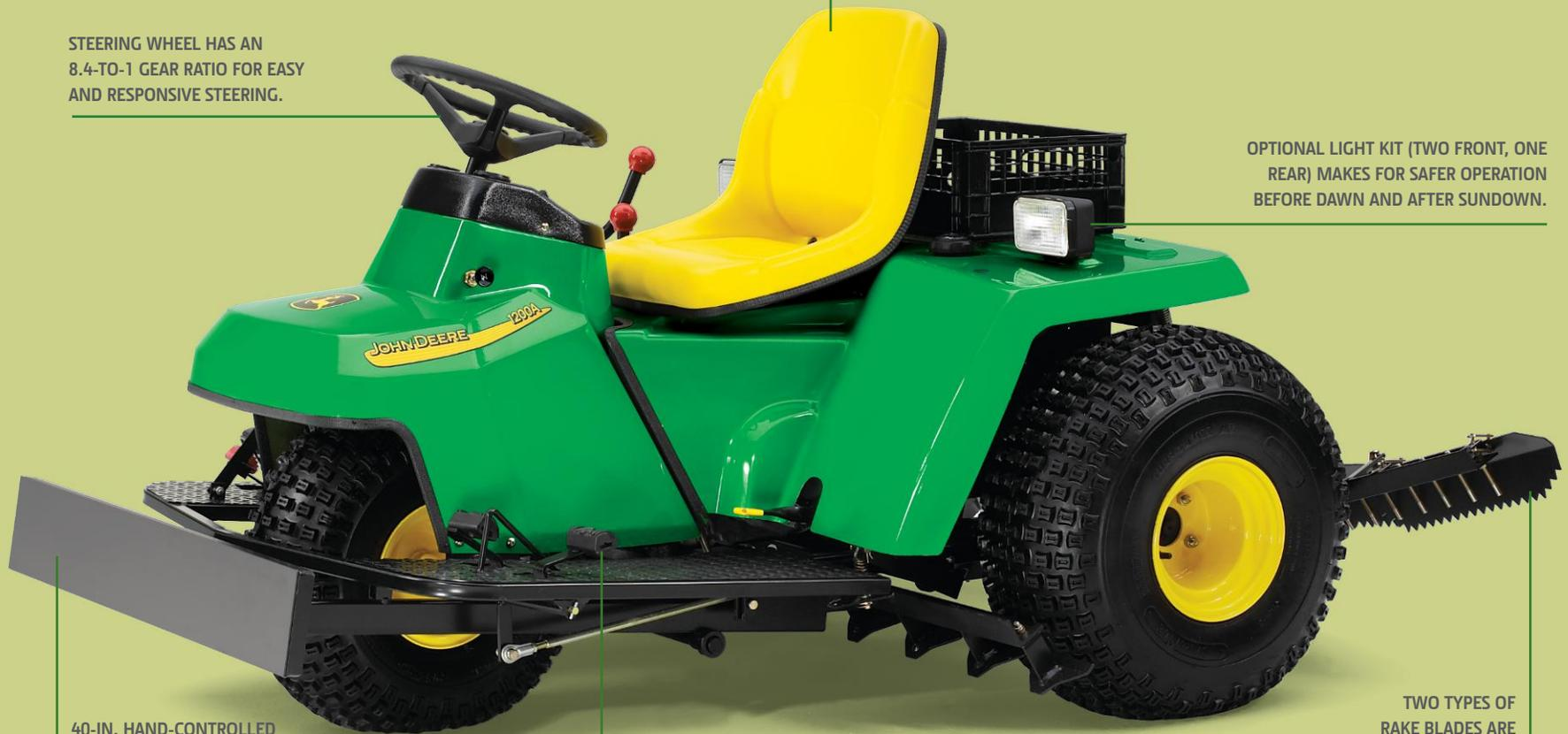
40-IN. HAND-CONTROLLED FRONT BLADE IS FABRICATED FOR YEARS OF SERVICE.
